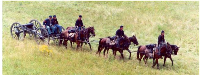
munition chest sat on top of the limber and provided a seat for cannoneers (above). The limbers were hauled by six horses although shortages, especially in the Confederacy, sometimes reduced the teams to four horses. Each cannon also had an additional limber to which was attached a caisson with two additional ammunition chests (below).
