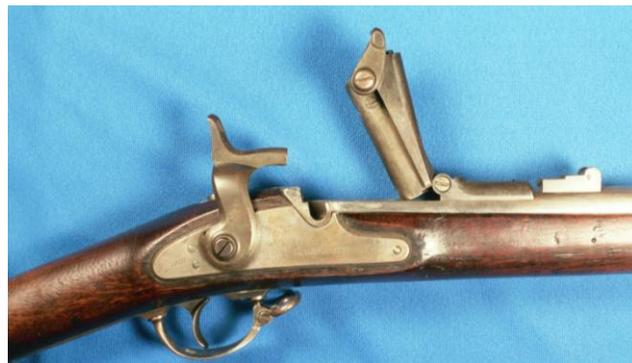
Model 1866 Rifle with open "trapdoor" converted from a M1863 Type II
